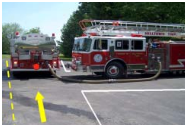
Figure 12. A “nose to tail” suction hook-up in which Tanker 61 supplies the quint through a gravity nurse operation with the tanker’s 28 ft of suction. In this particular operation, the quint backs into the driveway, to keep from blocking the road. Should a dump & run operation be needed, the suction hose can be disconnected from the tanker, and the porta-tank from Tanker 61 can be dropped in front of the quint so mutual-aid tankers can dump their water into the porta-tank. As additional tankers arrive, additional porta-tanks are set up and jet-siphons used to transfer water to the draft porta-tank.
