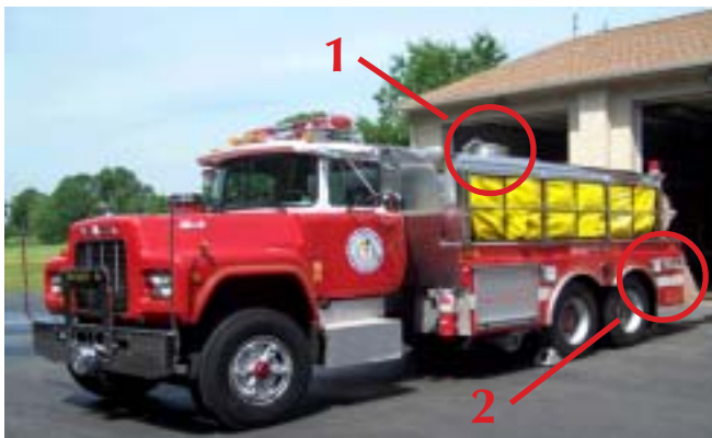
Figure 10. Tanker 61 carries a 3000-gal porta-tank, is equipped with a remote-operated over-sized vent (1) and exterior vent and dump valve controls (2) on the driver side as well as in the cab.
