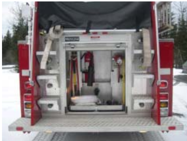
Figure 9. The rear compartment neatly houses portable extinguishers, hand tools, extra hose, a pike pole and the direct tank fill.
