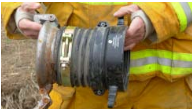
Figure 4. Elk Horn and neighboring department engines carry suction adapters from the irrigation pipe connection to fire department suction thread.
