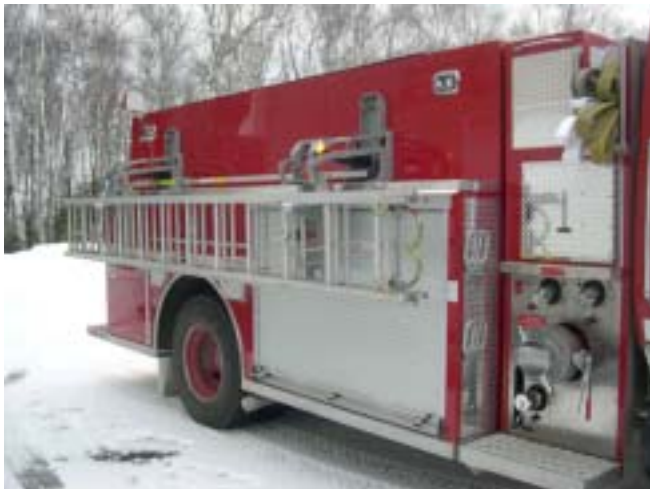
Figure 8. A ladder rack was installed in keeping with the concept of making equipment available within the reach of a normal person. Both 5" pump suction intakes are provided with butterfly valves for drafting operations.
