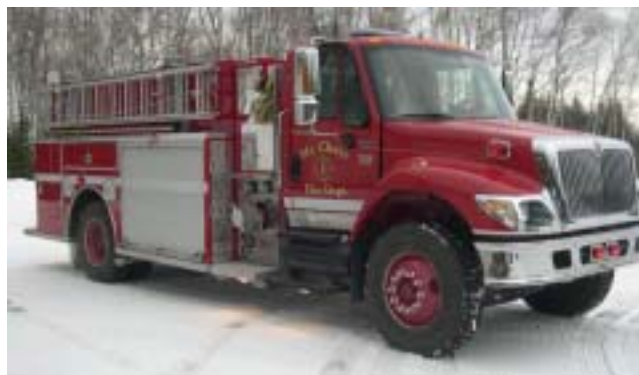
Figure 5. Mt. Chase VFD's $169,000 pumper is equipped with a 1000-gpm pump, a 1000-gal tank and an 80cfm compressed air foam system (CAFS).
