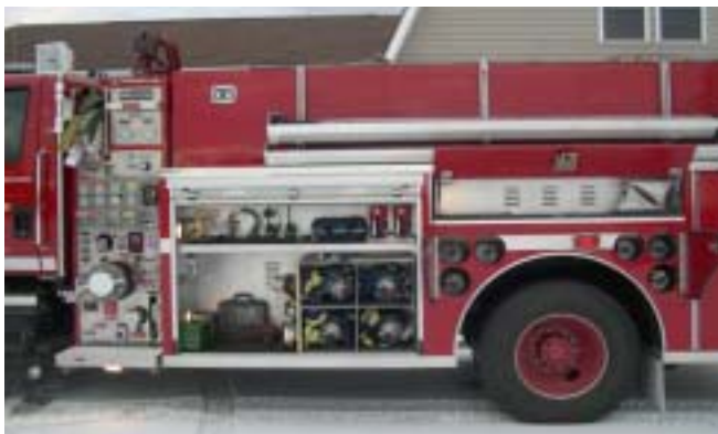
Figure 6. A narrow pump panel was used to reduce the apparatus length. Two 1-3/4" crosslay preconnects (1 piped with CAFS) and a pre-piped deck gun are provided. Four SCBA are stored horizontally to save space and the 6 spare SCBA cylinders are located on the driver's side.
