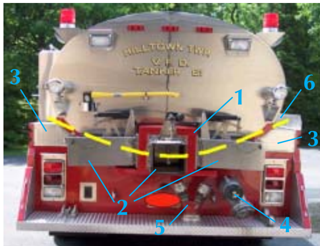
Figure 11. The “working end” of Tanker 61. A lot of attention was paid to the details in designing this tanker. Three electric 10” Newton dumps are connected to a distributor box (1) that sits well below the bottom of the tank (yellow line) and is connected to a 10° sloping trough cut into the length of the bottom of the tank to increase flow. Each dump has a 3-section manual extendable chutes (2). Two 14-ft lengths of 5” suction with Storz couplings are carried — one in each rear compartment (3) — for gravity nurse operations. A 5” pipe (4) serves as both the direct tank fill and as the suction hose connection for gravity nurse operations. A 3” Storz x 5” Storz siamese (5) is also carried. A jet-siphon for porta-tank water transfer is carried connected to a length of hard suction in a trough on the passenger side (6).
