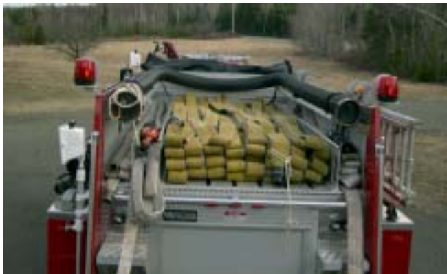
Figure 7. A 25-ft section of lightweight 5" suction is stored so one person can easily remove it and connect it. The hose bed carries 1200 ft of 3" supply line as well as additional 1-3/4" and 2-1/2" preconnects.
