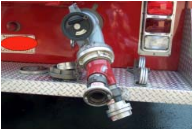
Figure 15. The 5" tank line is equipped with a piston-intake valve (with a 5" Storz connection). While county SOPs call for filling with a 5" line, the 3" x 5" siamese (shown attached) is carried for use in case dual 3" lines must be used because a 5" fill line is not available. Notice that Storz wrenches are carried at the point at which they are likely to be needed — simple things like this can help eliminate chaos.
