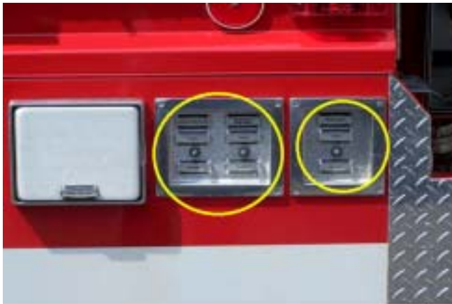
Figure 14. Dump valve controls are also located at the rear of the driver side (see Figure 10) for operation by the tanker spotter if needed.
